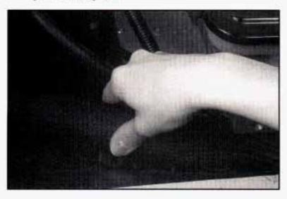
Start the engine and let it run until you can feel the upper radiator hose getting hot. Watch out for the engine fan. By this time the coolant level inside the radiator filler neck may be lower. If the level is lower, add more of the proper mix through the filler neck until the level reaches the base of the filler neck.
